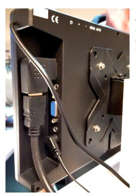
This image shows the video and power cables connected to the BlocDoc monitor. The cable running from the top of the monitor is a USB cable that facilitates the touch screen interface for the BlocDoc system.
