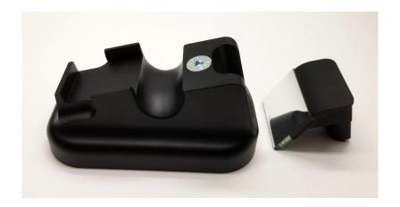
The sample holders have a magnetic mirror attachment that must be attached. When mounting the mirror it is ideal to slide it to the rear as much as possible. The correct orientation is shown below with a green arrow. The incorrect orientation is shown with a red arrow.
